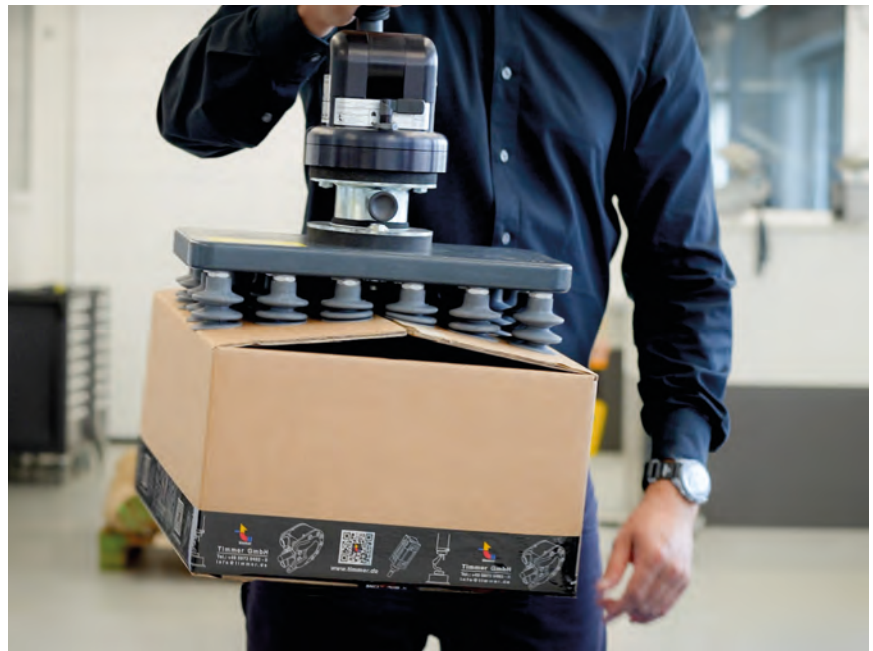
The vacuum hose lifters from Timmer improve ergonomics and efficiency in the workplace. 29 bellows suction cups ensure a wide range of applications.
